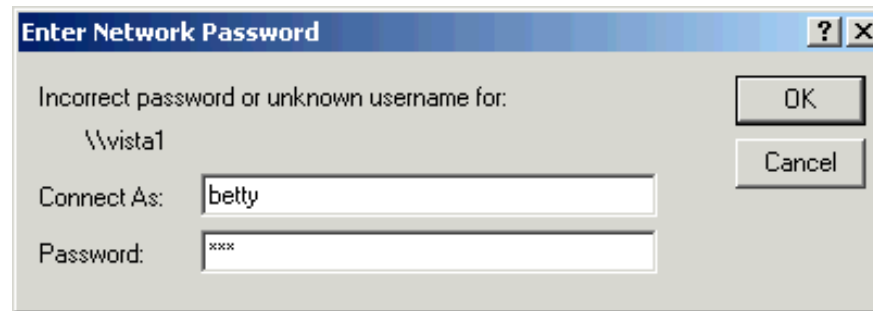
Figure 25. My logged-on name and password don't match one in the Vista box, so I need to enter a name/password combination it recognizes
