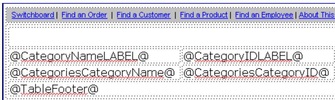
Figure 2. The tokens for the various portions of a list box (column labels, the data rows and a footer for the table). Note that this browse used a design time HTML file that had a navigation bar at the top.
