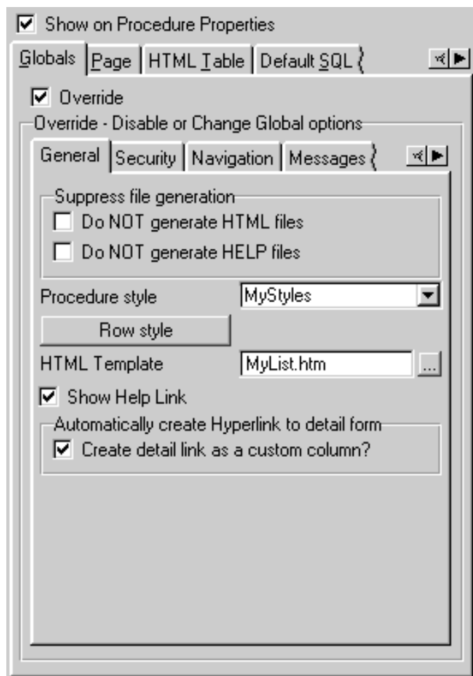
Figure 5. Overriding the global defaults on a single procedure. These options give you complete control of how this procedure will be generated, what design time HTML file will be used, which style sheet, text for prompts and much more.
