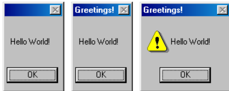
Figure 2. Using the message function passing one, two and three parameters respectively
